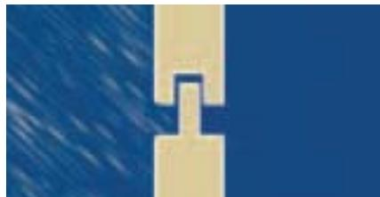
Figure 1.2: Proper Joinery Design Can Counteract the Forces That Drive Rainwater Into a Building.
